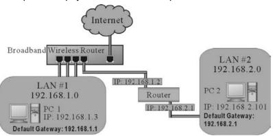
In the above diagram, PC2 in LAN#2 is connected to the Wireless Security Router via another router while PC1 in LAN#1 is connected to the Wireless Security Router directly. Without configuring the Static Routing function, the two PCs would not be able to communicate with each other.
