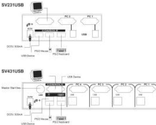
Figure 2: Console Connection
