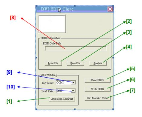
Ensure that power is connected and proper Com Port is selected. Then click on Auto Scan ComPort
