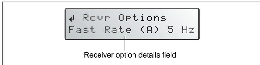
Figure 4.5 Example of a display-only field
