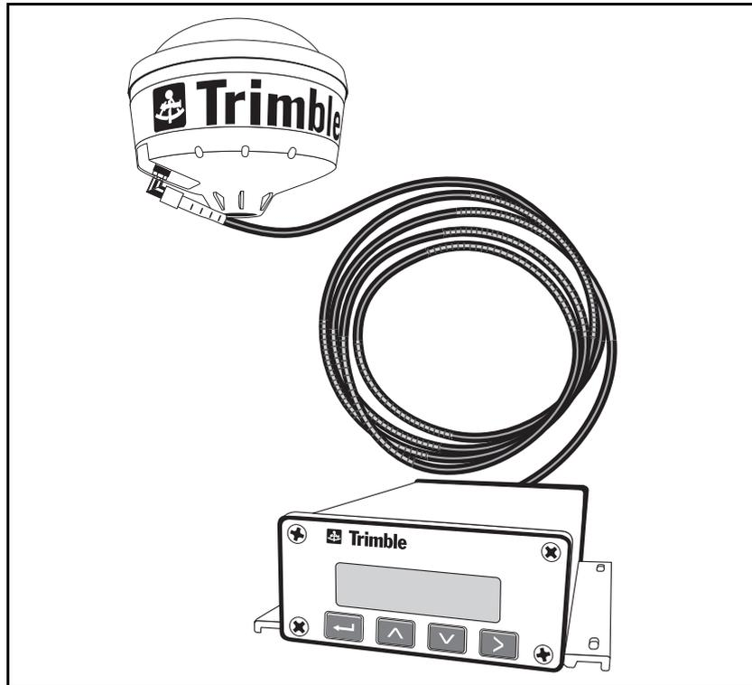
Figure 2.1 DSM 132 receiver
