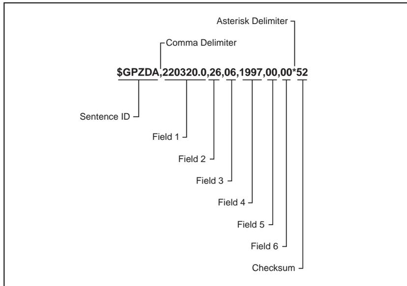
Figure C.5 Example showing NMEA-0183 message structure — ZDA
