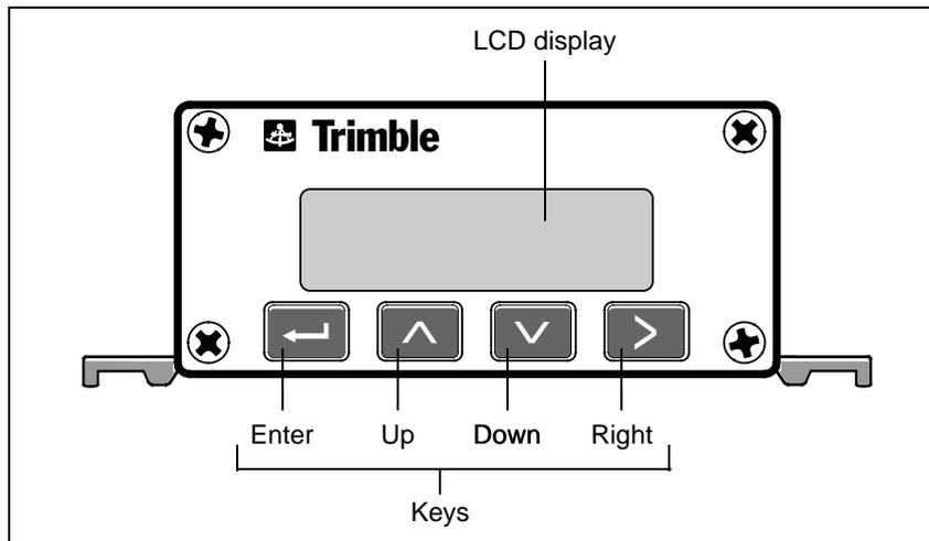
Figure 4.1 DSM 132 receiver front panel
