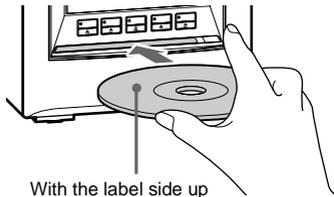
To load another disc, eject a disc or press one of the buttons (DISC 1 – 5) to select an empty compartment (it is not possible to select another compartment, when an 8 cm disc is loaded).
