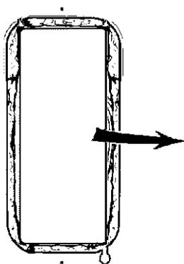
4. **Lower Element:** Lift out the tab as shown to unclip the terminal cover from the thermostat. The terminal cover can be removed from the thermostat.
