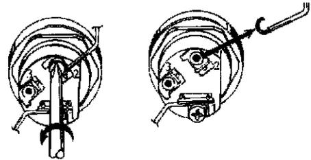
6. The buss bar is labeled 5500 W. Place the buss bar over terminals 2 and 3 with the 5500 W visible. Install the extra screw provided into terminal 3.
