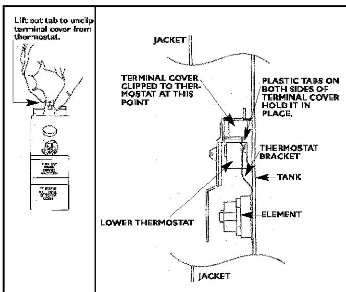
5. Remove the screws from terminal 2 of the element, and move the looped end of the wire aside.
