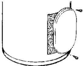
3. Remove the insulation block and pad.
