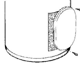
5. Remove the insulation block and pad.
