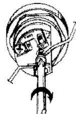
8. Tighten terminals 2 and 3 to ensure proper electrical connection.
