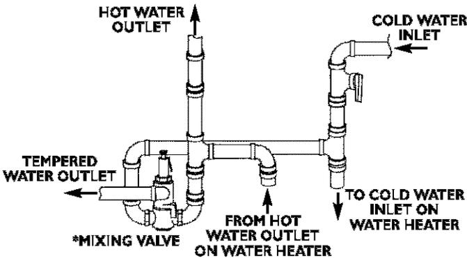
The illustration shows the attachment of the water piping to the water heater. The water heater is equipped with  $\frac{3}{4}$ " water connections.
