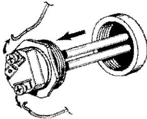
8. Clean the area around the element opening. Remove any sediment from or around the element opening and inside the tank.
