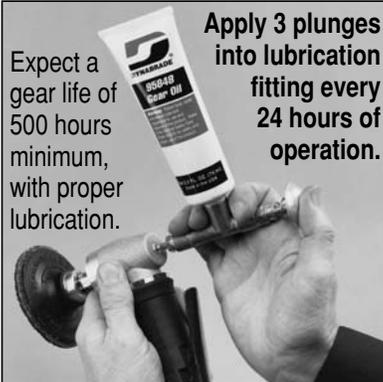
Lubricate wick system through the angle gear oil fitting with 2-3 plunges for every 24 hours of use, to achieve maximum gear life.
