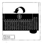
by turning the lever on the flap to the left – flap springs open.
