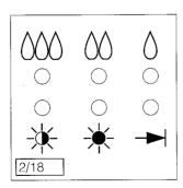
I feature an electronic programme stage indicator for programmes 1 − 8. As the laundry reaches a certain degree of dryness the relevant symbol lights up. On completion of the drying programme the end-of-programme symbol → also lights up.
