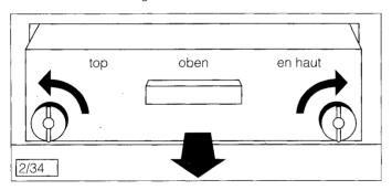
by turning the two locking discs a quarter turn in the direction of the arrows.
