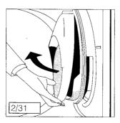
Fluff is more easily removed if you damp your hand slightly or use a damp cloth. After cleaning the fine filter, fold down and clip in coarse filter.
