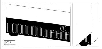
Even if the machine is built-under into a fitted kitchen the ventilation slots must be left open.
