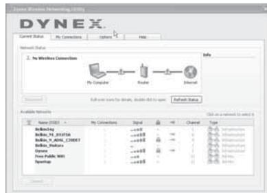
The WNU's default screen is the **Current Status** tab, which displays the current network status and available networks.
