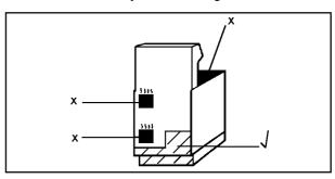
To move the appliance, open the main oven door, and lift the appliance by holding inside the top of the oven compartment.
