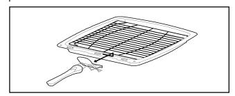
Place the grill pan on the shelf so that the pan is positioned centrally beneath the grill.
