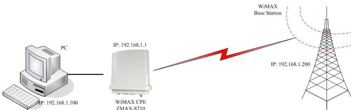
**Figure 11 Build the Infrastructure with WiMAX Base Station**
