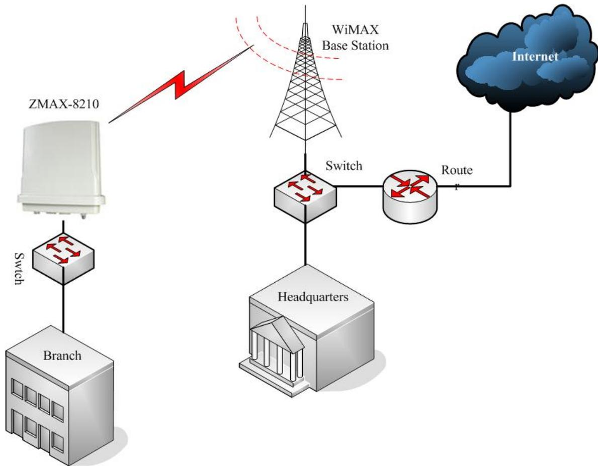
**Figure 3 Wireless Point-to-Point Outdoors**
