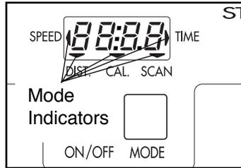
When the power is turned on, the SCAN mode will automatically be selected. One mode indicator (see the drawing above), will appear by the word SCAN, and a second mode indicator will show which mode is currently displayed.
