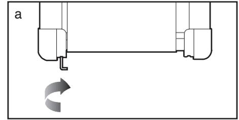
b. If the walking belt has shifted to the right, first remove the key and **UNPLUG THE POWER CORD**. Using the allen wrench, turn the rear roller adjustment bolt counterclockwise 1/4 of a turn. Plug in the power cord, insert the key and run the treadmill for a few minutes. Repeat until the walking belt is centered.
