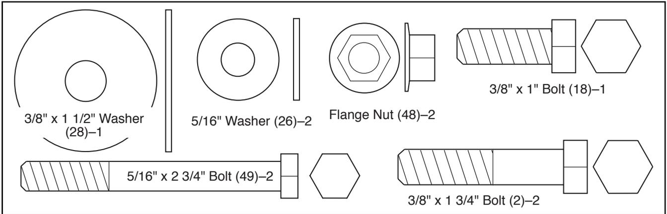
1. Raise the Upright (11) to the vertical position. Insert the 3/8" x 1" Bolt (18), with the 3/8" x 1 1/2" Washer (28), into the lower end of the Upright. Finger tighten the Bolt into the Frame (59).
