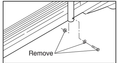
Remove the bolt from the upper end of each handrail.
