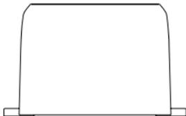
For best results, the rain sensor should be securely mounted onto a horizontal surface about 1 meter above the ground and in an open area away from trees or other coverings where rainfall may be reduced causing inaccurate readings.
