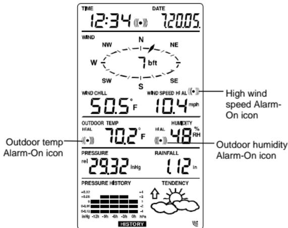
The Weather Center can be set to alert when a specific weather condition is reached.
