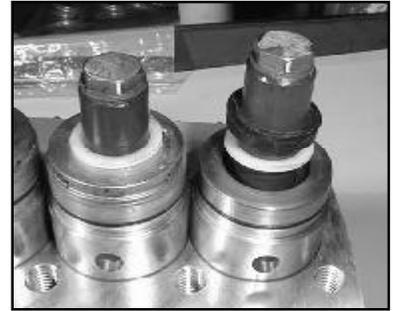
11) Place pressure rings and weep seals (23B) over plungers and into each seal case (20).
