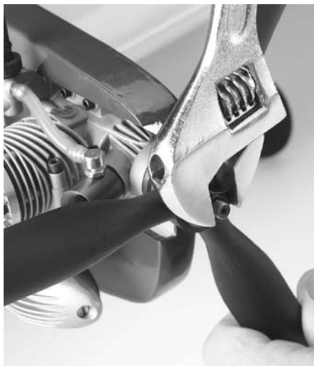
Securely tighten the prop nut using an adjustable wrench.
