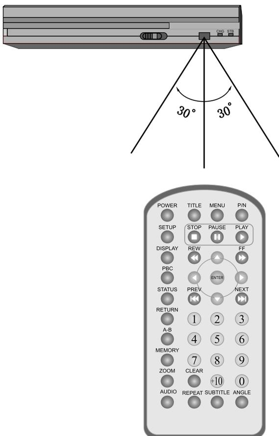
Do not expose the remote sensor of the unit to strong light source such as direct sunlight or other illumination.
