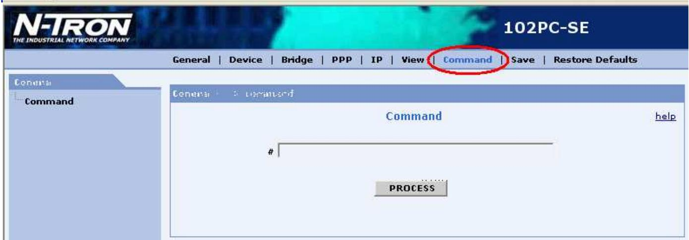
Don't forget to save the running configuration after making changes. Otherwise settings may not change after a power cycle on the switch.
