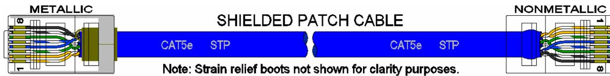
In the event all Cat5e patch cable distances are small (i.e. All Ethernet devices are located the same local cabinet and/or referenced to the same earth ground), it is permissible to use fully shielded cables terminated to chassis ground at both ends in systems void of low level analog signals.
