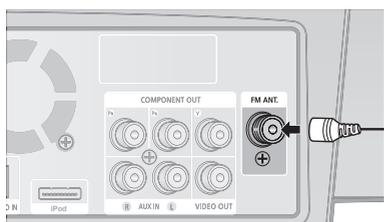
1. Connect the FM antenna supplied to the FM Antenna Jack.
