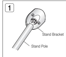
2. Insert and tighten three large screws (5x15, For connecting Stand Pole & Stand Bracket) into the three holes on the Stand Bracket as shown in the illustration.
