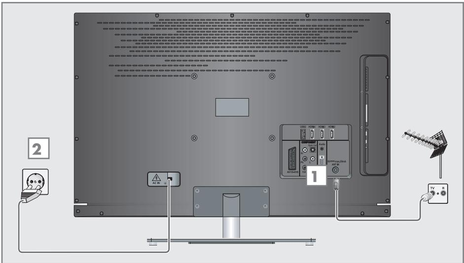
**1a** To receive terrestrial digital broadcasters (DVB-T) connect the cable for the rooftop or indoor antenna (passive or active indoor antenna with its own power supply) to the antenna socket »**ANT IN**« on the television set;
