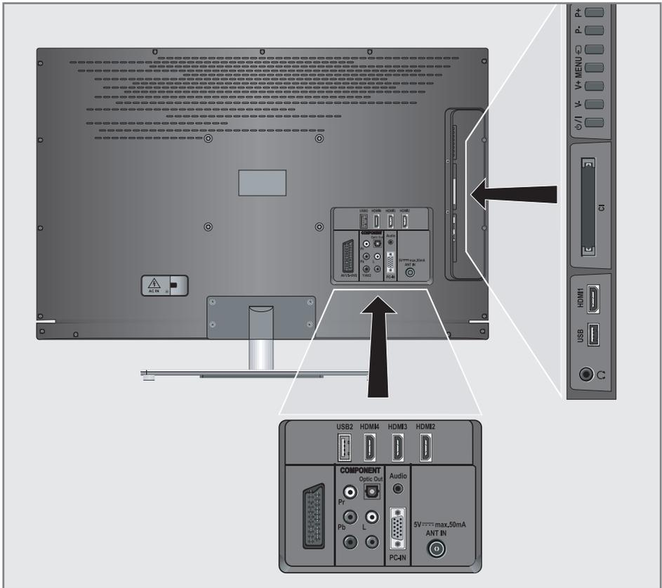
**AV1 / S-VHS** SCART socket (CVBS signal, RGB signal); Video and sound socket for S-Video camcorder.
