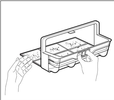
7. Use a moist hand to clean the filter. If necessary clean the filter with warm water using a brush. Close the filter.
