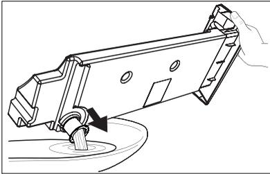
3. Move the plastic connection out and drain the water container into a sink or equivalent receptacle.
