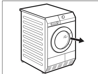
2. Pull 2 plastic hoses with the polystyrene blockages out from the drum.
