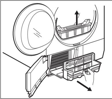
5. Lift the primary filter. Hold the heat exchanger filter and pull it out from the bottom compartment.
