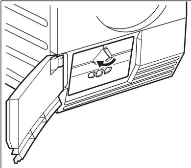
3. Turn the blockage to unlock the heat exchanger cover.
