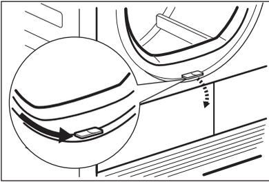
2. Move the release button on the bottom of the door opening and open the heat exchanger door.
