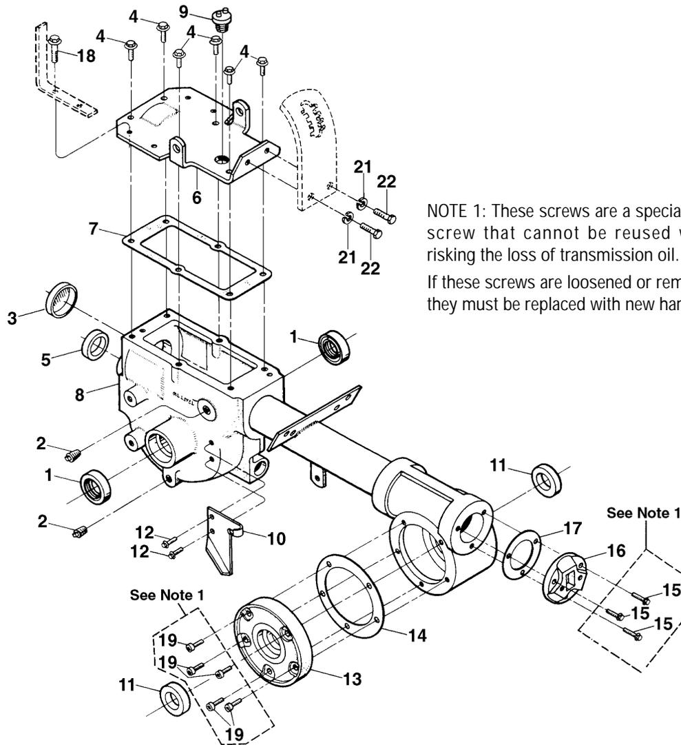
NOTE 1: These screws are a special sealing screw that cannot be reused without risking the loss of transmission oil. If these screws are loosened or removed, they must be replaced with new hardware.
