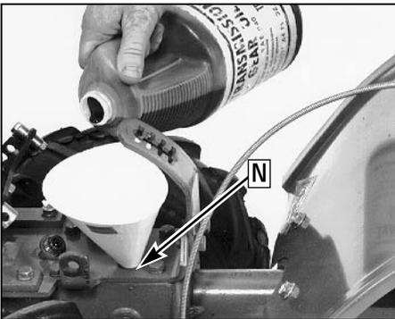
Figure 2-10: Adding gear oil.
