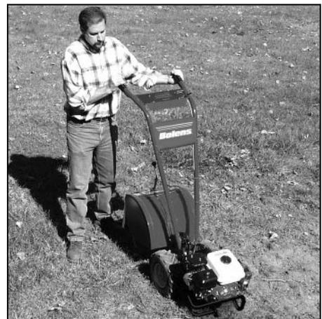
Figure 4-4: Push handlebars sideways to turn tiller.
