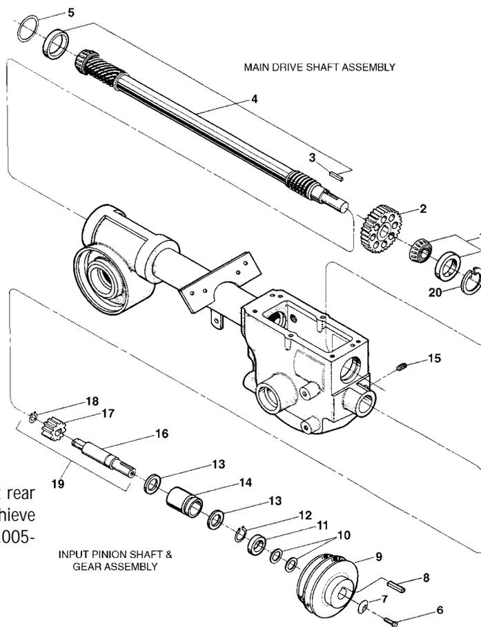
NOTE 1—Shim between drive shaft rear bearing and rear bearing cap to achieve 5-to-10 thousandths of an inch (.005-.010) end play on drive shaft.
