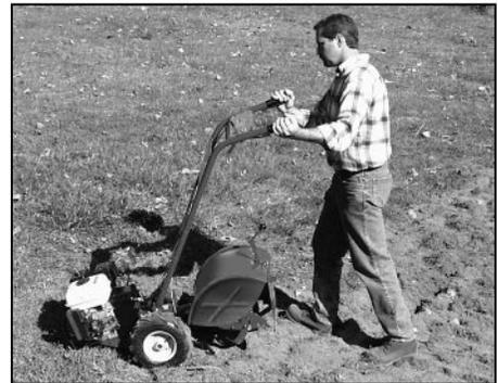
Figure 4-3: Find balance point before turning.
