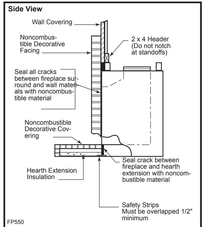
Fig. 25 Sealing gaps.
