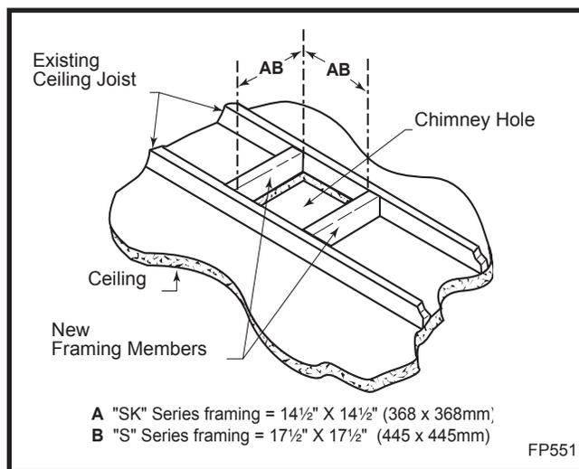
Fig. 12 Typical frame for ceiling chimney hole.
