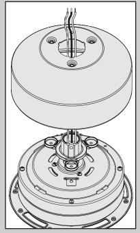
Thread the wires through the top housing.
