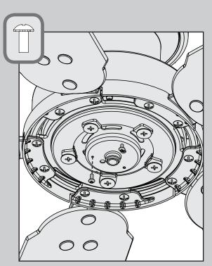
Screw two (2) housing assembly screws from the hardware ≡ bag halfway into the motor housing. It does not matter which two screw holes you choose.
