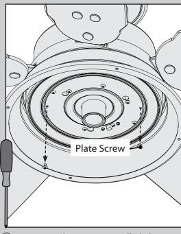
Remove the two pre-installed plate screws from the switch housing.
