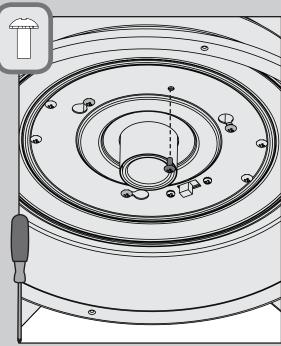
Remember the screw you saved? Install it back into the housing. Tighten all four screws firmly.
