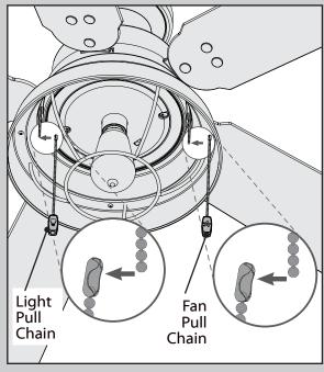
Connect the appropriate pull chain pendant to each of the short chains coming from the switch housing.
