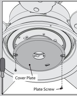
Lift the cover plate, aligning the screw holes with the screw holes in the switch housing. Install the plate screws to secure the cover plate to the switch housing.
