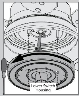
Align the keyhole slots in the lower switch housing with the stand off screws. Turn the housing counterclockwise until the standoff screws are firmly situated in the narrow end of the keyhole slots.
