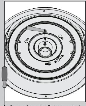
Remove the pre-installed screw and red label from the switch housing.
