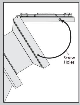
Swing the fan up to align the canopy screw holes with the mounting holes on the ceiling plate.
