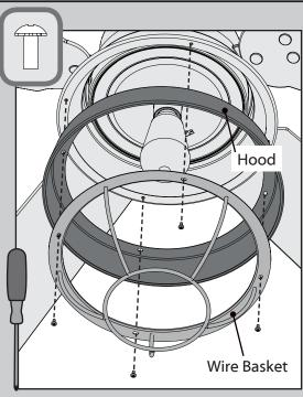
Align the holes in the wire basket and the hood with the holes on the rim of the upper switch housing. Install four switch housing screws, found in the hardware bag, through wire basket and hood into the upper switch housing.
