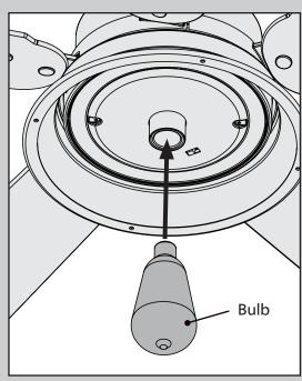
Install one E-26 60-watt light bulb. When necessary, replace with bulb of the same wattage.
