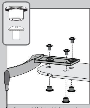
Secure each blade to a blade iron as shown 😵 using the blade nuts, found in the ■ hardware bag, and the blade assembly screws, found in the **A** hardware bag.
