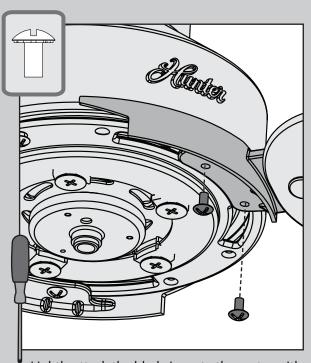
Lightly attach the blade irons to the motor with the blade iron armature screws, found in the X hardware bag, then securely tighten after all screws are attached.
