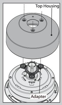
Place the top housing onto the motor housing so that the holes in the top housing lineup with the holes in the motor housing and the adapter.
