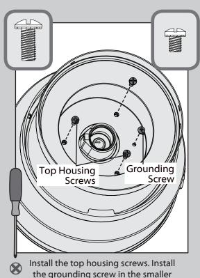
Install the top housing screws. Install the grounding screw in the smaller screw hole. These screws can be found in the hardware bag.
