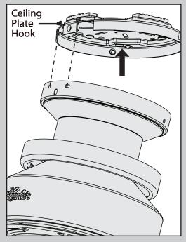
Raise the fan and align the slots in the canopy with the hooks on the ceiling plate.
