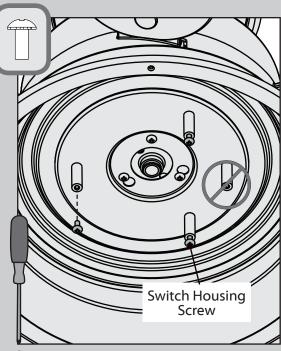
To attach the lower switch housing, partially install three switch housing screws into the standoffs as shown, leaving the circled standoff empty.
