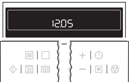
After about 5 seconds, the flashing stops and the clock displays the time of day set.
