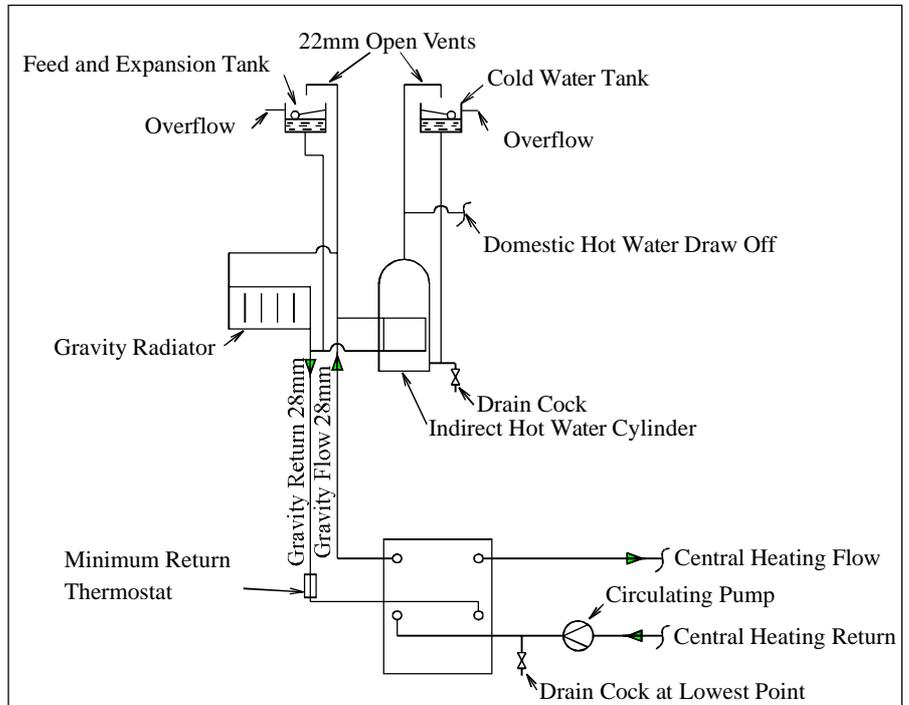
Fig. 5. Typical Central Heating & Hot Water System
