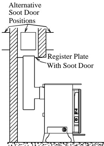
Fig 9. Horizontal Register Plate With Rear Flue Connection
