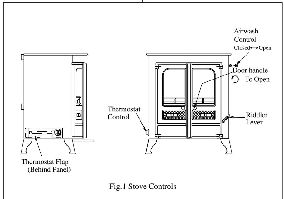
or fire lighters, and kindling on the grate and cover with approximately 2 inches of fuel. Turn the control knob to maximum, and open the airwash control fully (see Fig. 1). Light the paper or fire lighters. Close the doors until the fuel is well ignited then load with fuel and adjust the air controls to the required setting.
