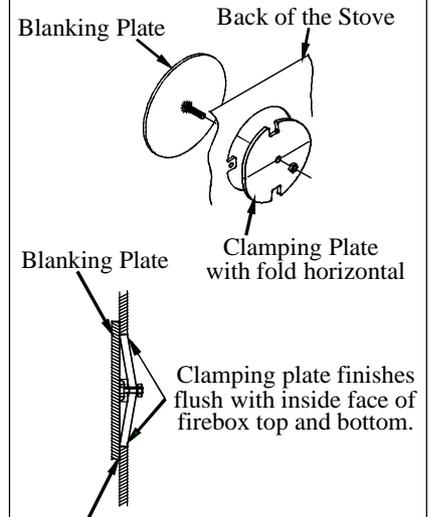
Fig. 12. Flue Blanking Plate.
