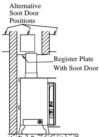
Fig 10. Horizontal Register Plate With Top Flue Connection
