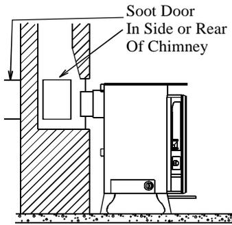
Fig 8. Vertical Register Plate With Bricked Up Fireplace
