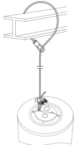
Seismic Tether for
