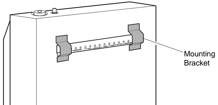
**Figure 6 - Mounting Bracket**
