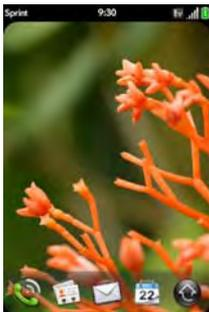
When you are inside a coverage area, the bars on the **signal-strength**
