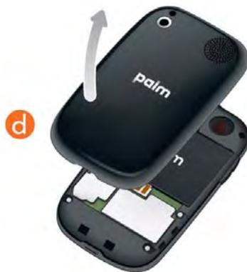
5. Remove the **battery** by pulling the tab that appears at the top of the battery.
