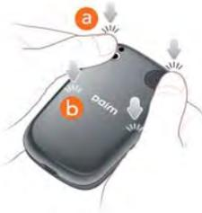
2. Slide out the keyboard (see “Slide Out the Keyboard” on page 31), and then press the two clasps at the bottom corners.
