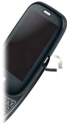
2. Connect the small end of the *USB cable* to the *charger/microUSB connector*.
