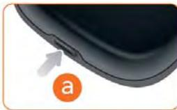
2. Slide your thumbnail or a credit card between the back cover and the phone, starting at the bottom and moving halfway up one side until you hear the clasp release.
