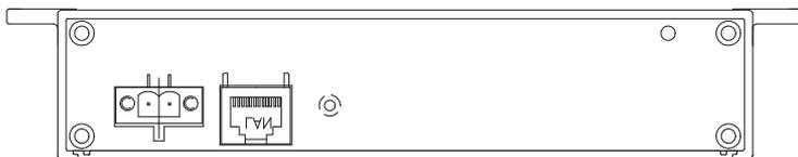
Figure 2-12 EDG-4504—Front Panel
