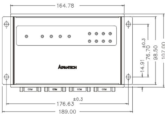
Figure 2-11 EDG-4504—Front Panel
