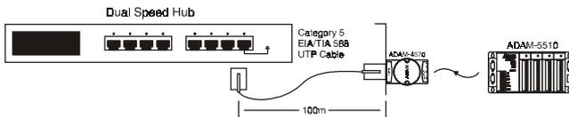
Figure 2-18 Connecting ADAM-4570/ADAM-4571/EDG-4504 series to the hub
