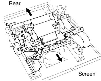
\* The stop position of the Scan Table should be set toward the rear for symptom 1 explained above and toward the screen for symptom 2.
