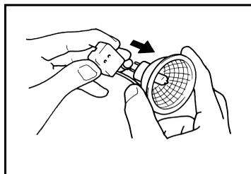
4 Insert a new Projection Lamp so that the mark on its base is facing upwards. Make sure that the new Projection Lamp is inserted securely so that there is no gap between the projection Lamp and the Lamp Socket.
