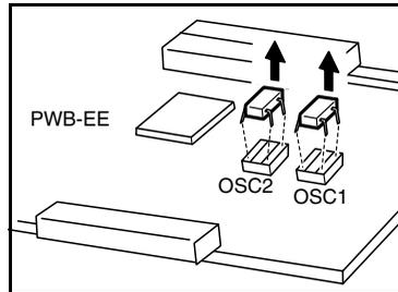
6 Install the Oscillator Chip supplied into the OSC1 socket as shown on
