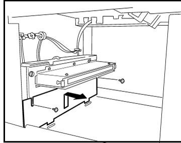
**4** Remove the front and rear Shield
