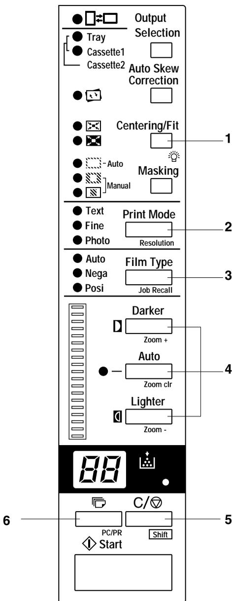
1. Lamp Illuminance Key: When this key is pressed together with the Shift Key, the illumination of the screen is adjusted. When this key is continuously pressed, the screen is gradually darkened until it is turned OFF. When any key is pressed then, the illumination returns to the maximum level.
