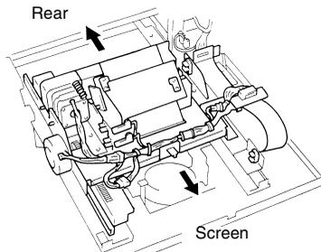
\* The stop position of the Scan Table should be set toward the screen for symptom 1 explained above and toward the rear for symptom 2.
