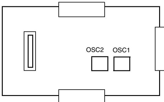
OSC1 ...Oscillator (42.3158MHz): For 400dpi Printer
