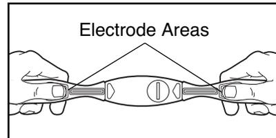
Next, hold the chest pulse sensor near the console. While holding one thumb stationary, begin tapping the other thumb against the electrode area at a rate of about one tap per second. Check the heart rate reading on the console.
