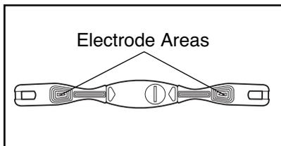
a saline solution such as saliva or contact lens solution, wet both electrode areas. Then, return the sensor unit to a position against your chest.
