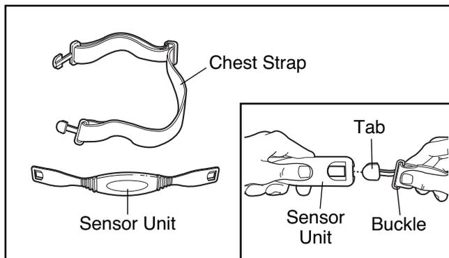
**See the inset drawing above.** Insert the tab on one end of the chest strap through the hole in one end of the sensor unit as shown. Make sure that the tab is flush with the sensor unit.
