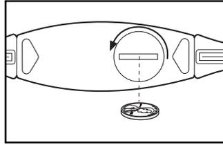
Remove the old battery and insert a new CR 2032 battery. **Make sure that the battery is turned so the writing is on top.** Reattach the battery cover and turn it clockwise to close it.
