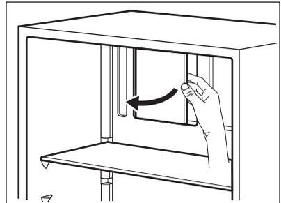
3. Insert the filter in the slot found in the back of the air lever flap.
