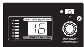
Fig. 3.1: Digital effects module (only X1204USB)
