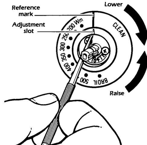
3. Put the blade of a small flat screwdriver into the slot of the temperature dial.
