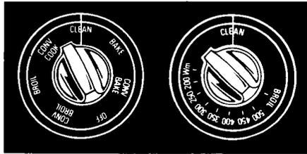
3. Set the Selector to CLEAN and turn the Temperature Control fully clockwise to CLEAN.
