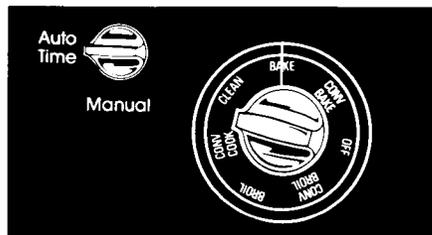
May be automatically timed to bake, roast, convection bake, convection roast and convection cook. The Selector for the upper oven will be set at one of these settings and the Auto Time switch set to AUTO TIME.
