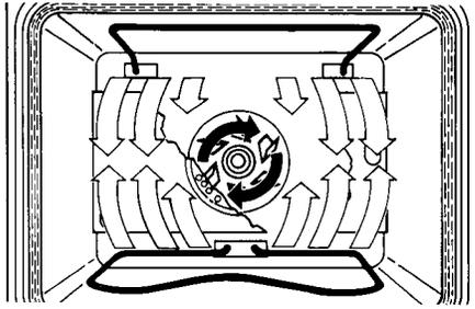
**CONVECTION BAKE** – The bottom element and outer top element operate at full power and glow red whenever heating. Air in the oven cavity is circulated by the fan for even heating and faster cooking. Use this setting for baking and roasting.
