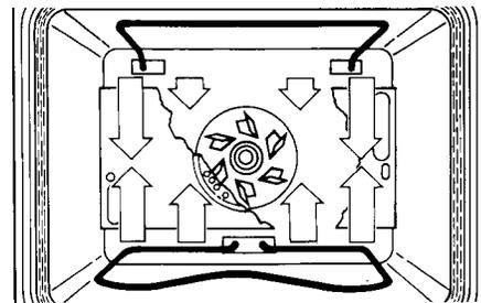
**BAKE** – The bottom element and outer top element operate at full power and glow red whenever heating. Use this setting for baking, roasting and casseroles.
