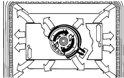
**CONVECTION COOK** – The rear element operates at full power whenever heating. Air in the oven cavity is circulated by the fan for even heating. Use this setting for foods which require gentle cooking such as pastries and souffles, and for baking yeast breads, quick breads and cakes. This setting is also recommended when baking large quantities of baked goods at one time.
