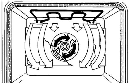
**CONVECTION BROIL** – The top element(s), as set by the Econo/Maxi Broil Knob, operate at full power whenever heating. Air in the oven cavity is circulated by the fan for even heating with the same results as a rotisserie. Use this setting for broiling thick cuts of meat.
