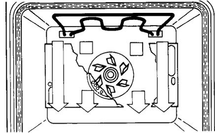
**BROIL** – The top element(s), as set by the Econo/Maxi Broil Knob, operate at full power whenever heating. Use this setting for broiling.
