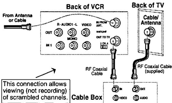
This connection allows viewing (not recording) of scrambled channels.
