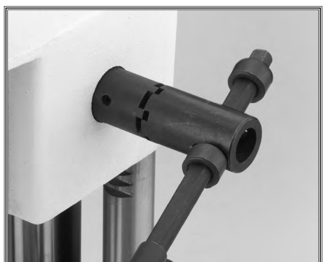
Fig. 6A. Secure depth stop before adjusting quick-set handle above. See Fig. 4.
