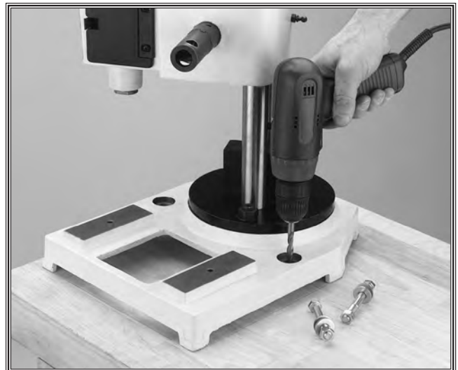
Figure 10. Using mounting holes as drill guides.
