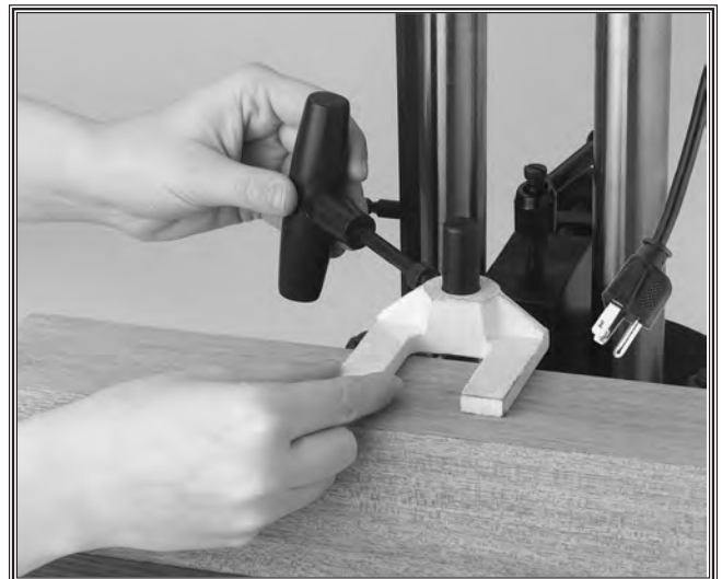
Figure 3. Always clamp workpiece.
