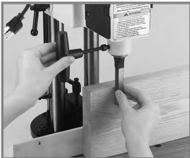
Figure 20. Back edge of chisel parallel with fence.
