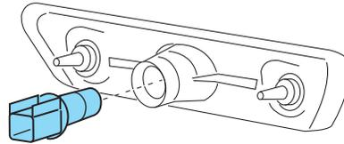
3. Rotate the socket counterclockwise and remove from the lamp assembly.
