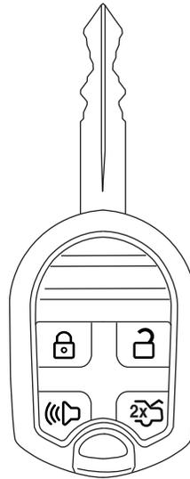
Your IKTs are programmed to your vehicle; using a non-programmed key will not permit your vehicle to start. If you lose your authorized dealer supplied IKTs, replacement IKTs are available through your authorized dealer. Standard SecuriLock® keys without remote entry transmitter functionality can also be purchased from your authorized dealer if desired.
