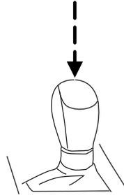
**Note:** The gearshift lever can only be moved to R (Reverse) by pushing the knob down before shifting to reverse. This is a lockout feature which protects the transmission from accidentally engaging R (Reverse) when intending to select 1 (First).
