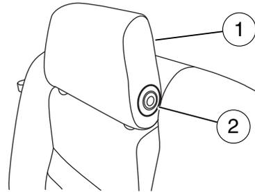
Properly adjust the head restraint to an upright driving/riding position by lifting up on the head restraint until it locks into its original position.
