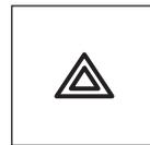
Press the flasher control and all front and rear direction signals will flash. Press the flasher control again to turn them off. Use it when your vehicle is disabled and is creating a safety hazard for other motorists.
