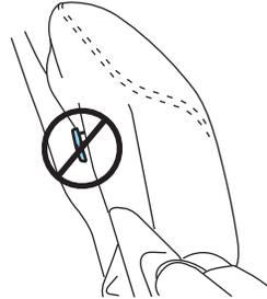
2. Access tether anchors located behind the seatback under the vinyl tag marked with the child tether anchor symbol.
