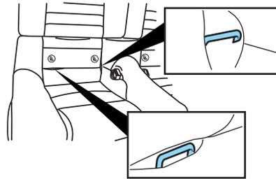
**WARNING:** The center of the rear seat is **NOT** designed as a seating position and is not equipped with safety belts. The LATCH anchors were not designed to be used with a child seat in the center position and there is no tether anchor available at the center. Attempted use of the center as a seating position will increase the risk of injury or death in the event of a collision.
