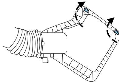
1. Release the clamps that secure the air filter housing cover.
