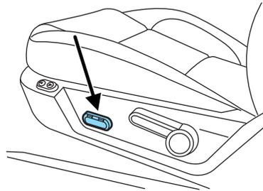
Move the switch in the direction of the arrows to raise or lower the front portion of the seat cushion.
