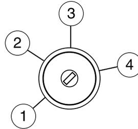
**Note:** Cranking may be stopped at any time by turning the key to the off position.
