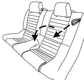
When raising the seatback(s), make sure you hear the seat latch into place. Pull down on the seatback to ensure that it has latched.
