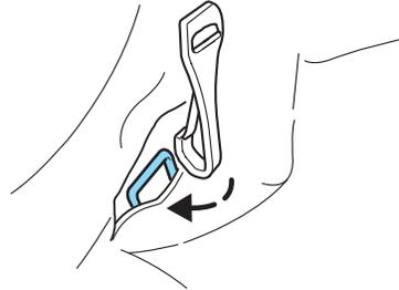
4. Tighten the child safety seat tether strap according to the manufacturer's instructions.
