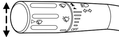
The flash rate of the turn signal indicator will speed up considerably if any of the turn signal lamps are out.
