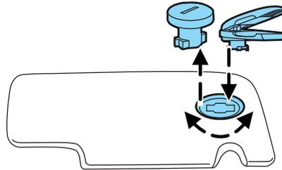
2. Insert the end of the storage accessory into the visor opening and turn 1/4-turn in either direction until the accessory snaps into place. For best results, ensure the open end of the accessory is facing away from the windshield.
