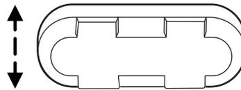
Move the switch in the direction of the arrows to raise or lower the rear portion of the seat cushion.
