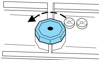
3. Note: For vehicles equipped with a V6 engine, the correct manual transmission fill level is at the lower edge of the filler hole. For vehicles equipped with a V8 engine, the correct manual transmission fill level is 1/2 inch (1.3 cm) below the edge of the filler hole.
