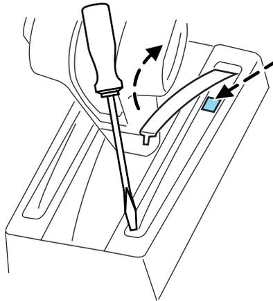
If it is necessary to use the above procedure to move the gearshift lever, it is possible that a fuse has blown or the vehicle's brake lamps are not operating properly. Refer to *Fuses and relays* in the *Roadside Emergencies* chapter.
