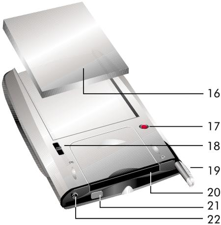
16. Main battery. Recharge the lithium-polymer main battery by connecting to ac power.
