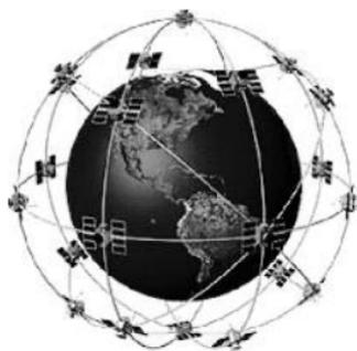
GPS uses a constellation of over 24 satellites that continually send radio signals to the earth. Your present position is determined by receiving signals from up to 16 satellites and measuring the distance from the satellites.
