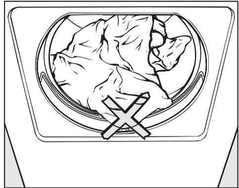
Check the laundry is right inside the drum so that it cannot get trapped or damaged when the door is shut.
