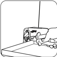
Pull out the emergency emptying cap from the filter cover, using a pliers.
