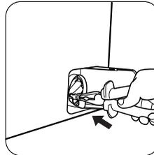
Replace the emergency emptying cap into the filter cover and fix it firmly.
