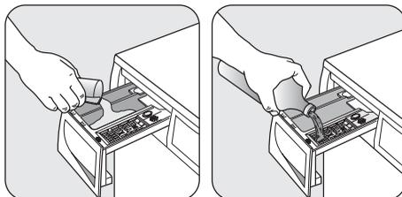
Pull out the dispenser drawer until it stops. Measure out the amount of detergent required, pour it into the main wash compartment
