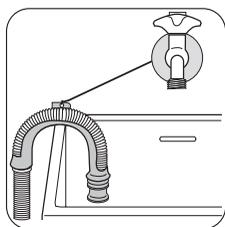
**Hooked over the edge of a sink using the plastic hose guide supplied with the machine.**
