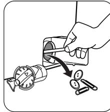
Remove any objects from the pump impeller by rotating it.
