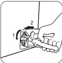
When no more water comes out, unscrew the pump cover, using a pliers, and remove the filter. Always keep a rag nearby to dry up spillage of water when removing the cover.
