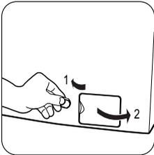
Open the pump door levering on the groove with a coin (or with the suitable tool, that you can find in the bag containing the instruction booklet, depending on the model).
