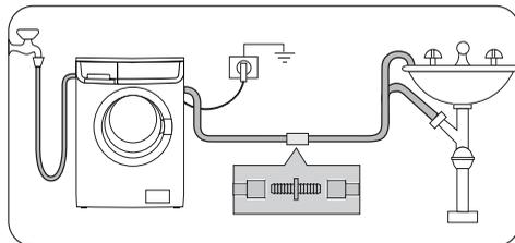
**In a sink drain pipe branch.** This branch must be above the trap so that the bend is at least 60 cm above the ground.
