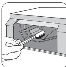
Having removed the drawer, use a small brush to clean the recess, ensuring that all washing powder residue is removed from the upper and lower part of the recess.
