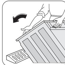
After removing all the packaging, carefully lay machine on it's back to remove the transit bolts from the bottom.
