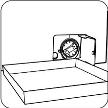
Place a bowl with a small edge close to the pump to collect any spillage.
