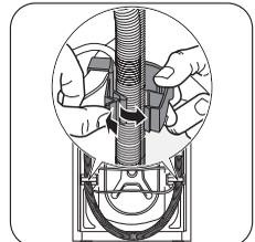
Remove the power supply cable and the hoses from the hose holders on the rear of the appliance.
