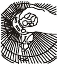
Secure the back grill by screwing on the mounting nut. Turn clockwise and tighten firmly.
