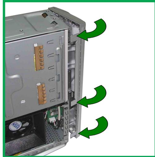
2. Align chassis cover tabs and push chassis cover towards the front panel.
