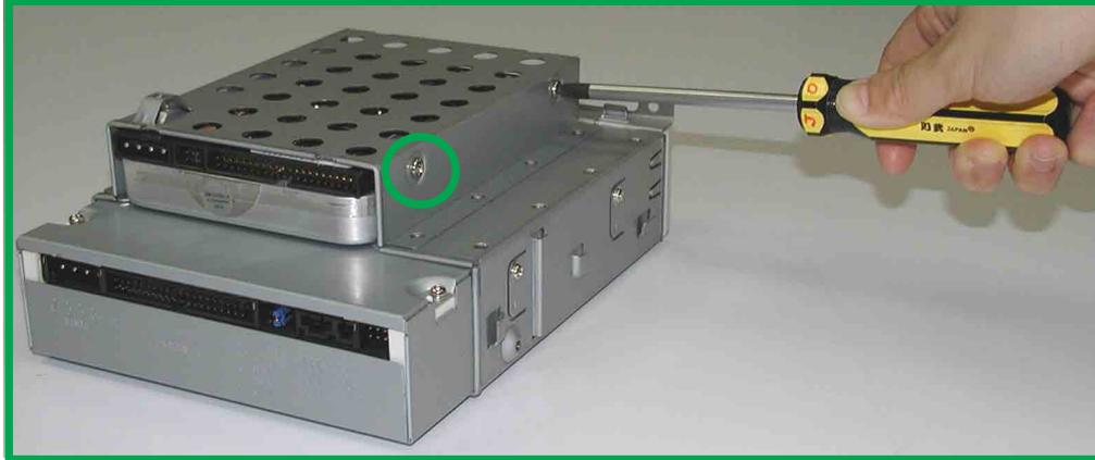
2. Slide the disk drive assembly back into its original place. Connect the middle connector of the IDE cable to the primary IDE connector on the hard disk drive. Locate the P5 power cable and connect it to the hard disk drive.
