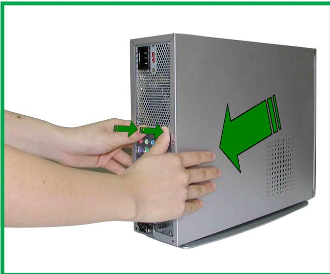
2. Separate the case and chassis cover: use your thumbs to pull it off, from the front to the back, then lift it off the chassis.
