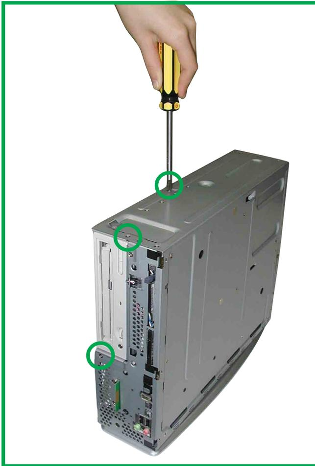
1. Remove the three screws on each marked location as shown. This frees the DVD/CD/HD drive assembly.
