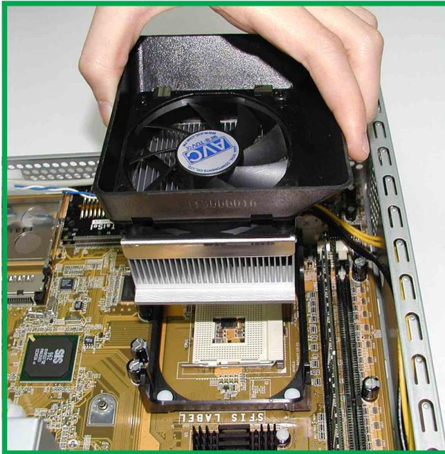
1. To install the CPU, it is necessary to remove the pre-installed heatsink assembly.
