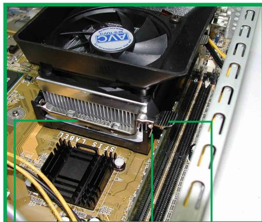
Retention bracket    Hole on the retention module    Locking lever
