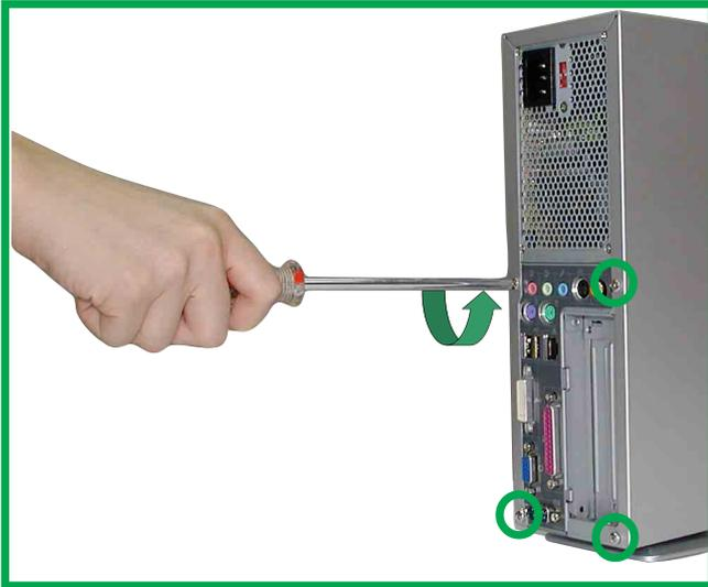
1. Remove the four screws on each end of the back panel. This frees the the chassis cover.
