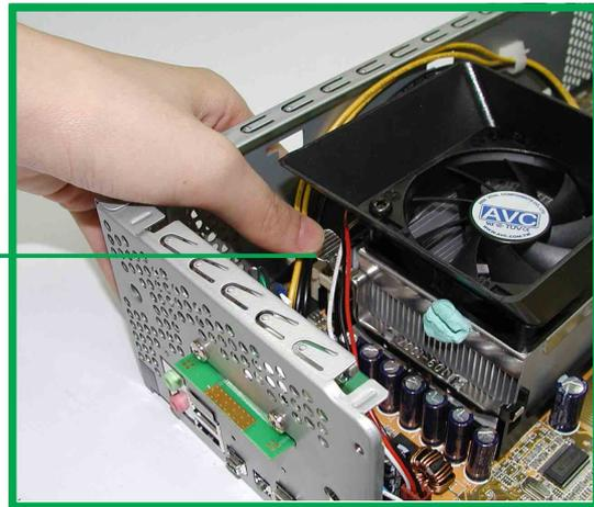
7. Connect the CPU fan cable from the assembly to the fan connector labeled CPU\_FAN1.
