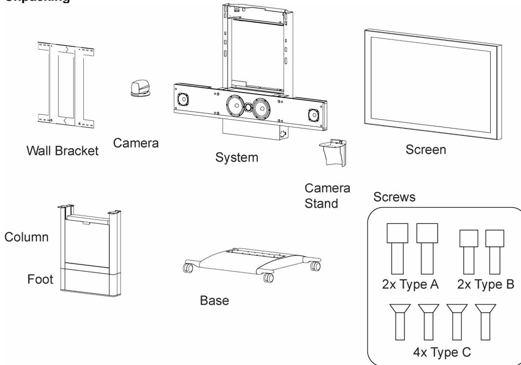
To avoid damage to the unit during transportation the system is delivered as separate components:
