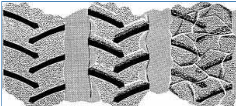
TOO MUCH BALLAST
