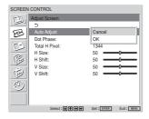
(2) Select "OK" with **↑**/**↓** and press ENTER. All the items of "Adjust screen" menu are adjusted automatically.
