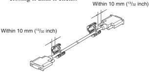
**2** Wind the stopper around the cable so that the ferrite core does not slide.
