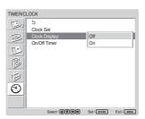
2 Select "On" with ↑/↓, then press ENTER. When you hide the menu, the clock appears on the lower right corner of the screen.
