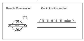
Operation of the unit is explained in these operating instructions for the case of operation using the Remote Commander. The  $\uparrow/\downarrow$  and ENTER buttons on the Remote Commander have the same functions as the  $\uparrow/\downarrow$  and ENTER buttons on the display.
