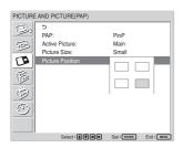
2 Adjust the position of the inset picture with **↑**/**↓**/ **←**/**→**, then press ENTER.
