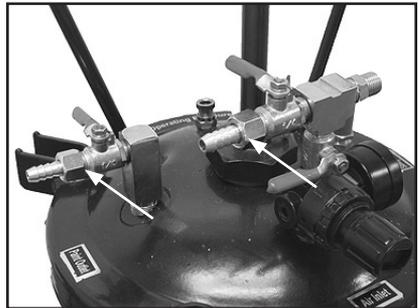
Figure 4. Spray gun fittings installed.
