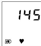
When the pressure lowers by 15mmHg after pressurization stops, the mark of "♥" lights up.
