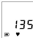
If the pulse is recognized, the pressure is shifted to the diastolic blood pressure display section and changed over, synchronized with the pulse.
