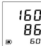
The buzzer sounds for two seconds, then the systolic blood pressure, diastolic blood pressure and pulse are indicated and the air is discharged. The measured data are registered automatically, as long as they are not error. If the measured data do not need to be stored, press the memory clear switch for 1 seconds or more while the measured data are indicated.
