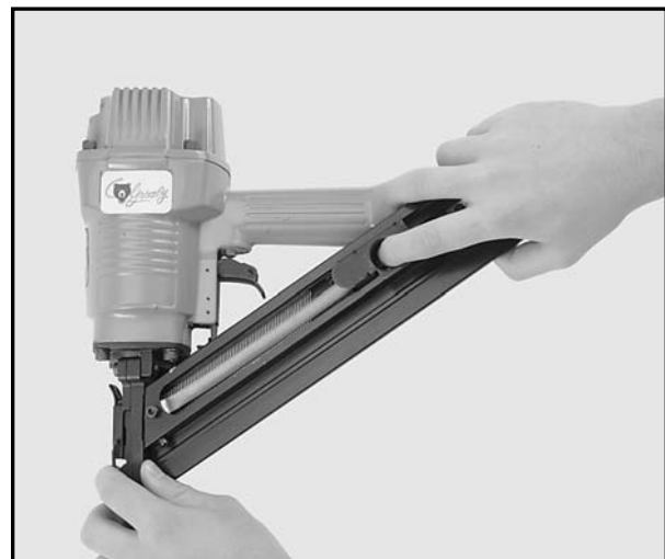
Figure 4 shows pulling back the spring handle to secure the nails and add pressure.
