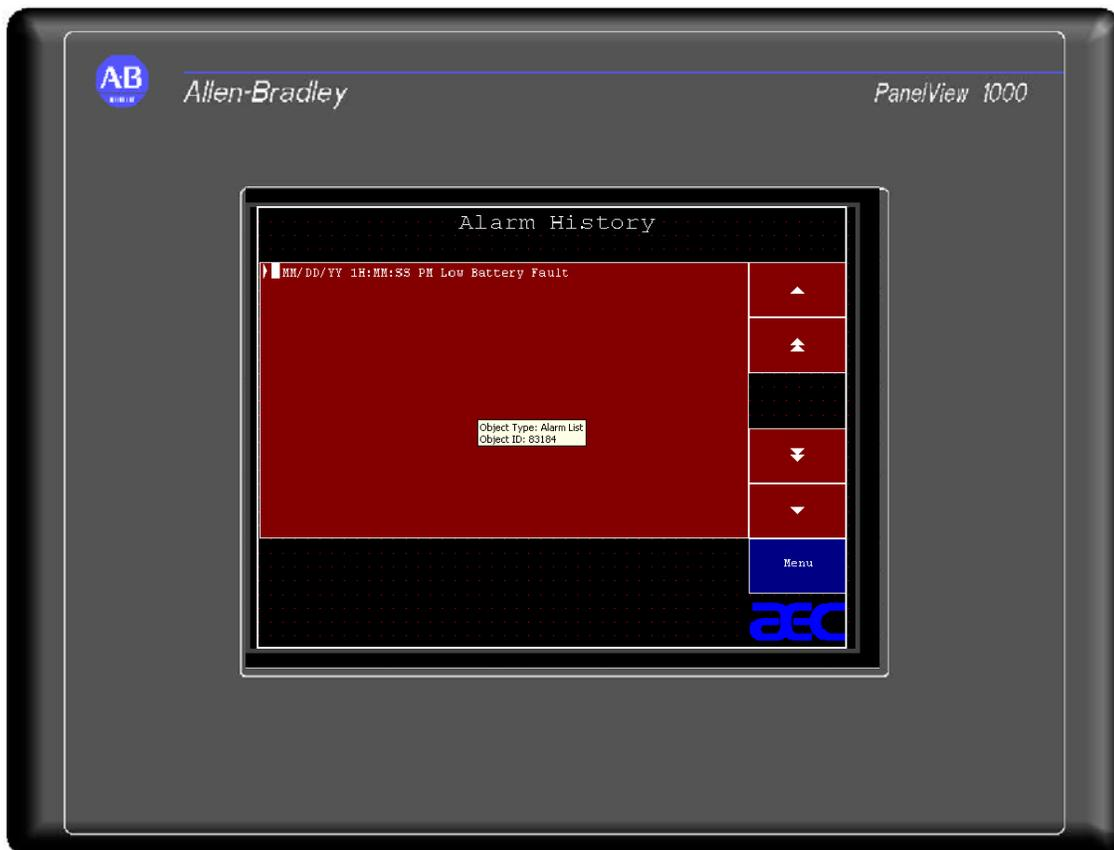
To acknowledge the alarm, press the alarm silence button to clear it. It will then appear in the alarm history screen. Except for High and Low Water Temperature, and Low Refrigerant Pressure, these alarms are considered fatal and maintenance must be preformed in order to allow the chiller to fully run. Should a compressor or pump turn off from an alarm condition, the remaining will shut down and display **FAULT** in the status screen for the device.
