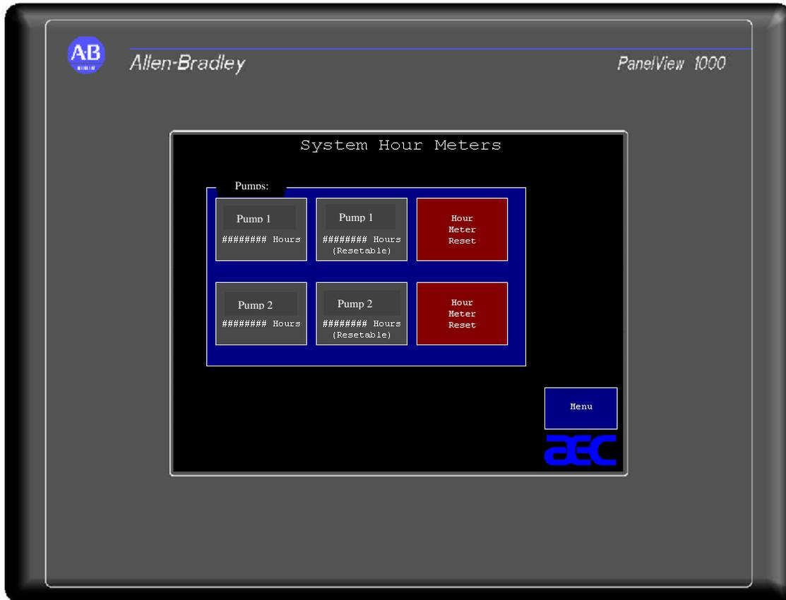
Two hourmeters are kept for each pump in the system. The first is a lifetime meter. This measures the total time that the pump has been operational in the lifetime of the chiller. The second is a resettable hourmeter. This hourmeter can be cleared to monitor run time on specific intervals. In order to clear the resettable hourmeter, press the appropriate “**Hour Meter Reset**” button (as prompted on the screen)
