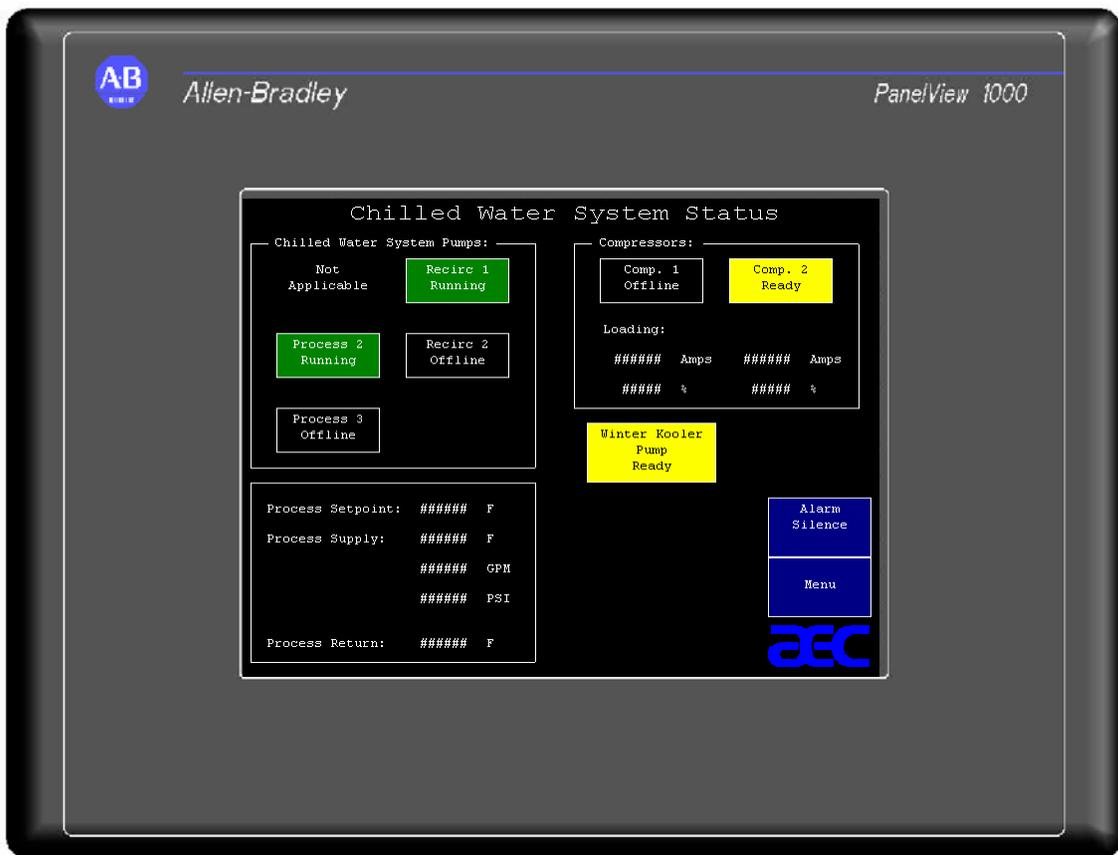
The Chiller Status screen shows the status for compressors within the system. Only compressors that are included in the system will
